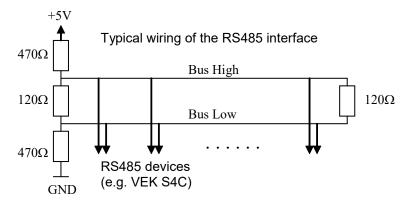
The shown resistors are switchable by the help of the DIP-switches
