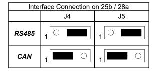
Both jumpers may be inserted only together for CAN or for RS485!
