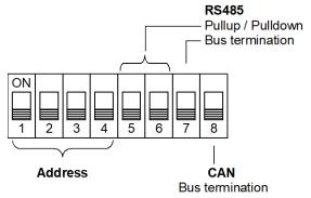
DIP-Switch address is only valid, if no address on DIN-connector is coded!
